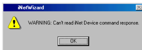
Figure 5B. WARNING indicating an incorrect command has been sent from iNetWizard® to the iNet device.
